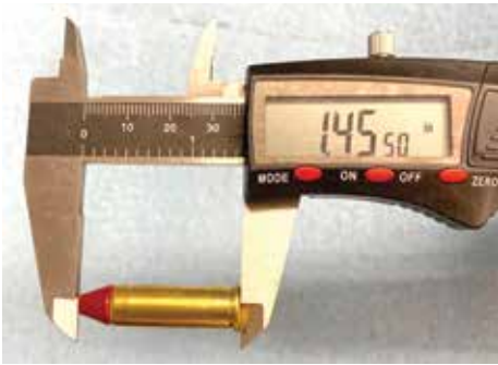
105-GRAIN TRUNCATED CONE BULLETS CAN BE LOADED FROM 1.44" TO 1.46" COL WITH THE CRIMP IN THE CRIMPING GROOVE. IF THE ROUND IS TOO SHORT, IT WILL ALLOW ENOUGH OF THE NEXT ROUND INTO THE LIFTER TO LOCK THE LIFTER.
