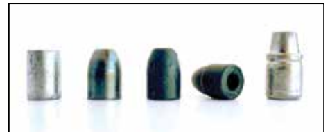
STEPS TO MAKING A BULLET (FROM THE LEFT): A CAST SLUG, A PRESSURE-FORMED BULLET MADE FROM THE SLUG (APPEARS DARK BECAUSE IT HAS BEEN TUMBLERED), A COATED BULLET, A COATED HOLLOW-BASE BULLET, A MOLDED BULLET WITH A CANNELURE AND A TRUNCATED FLAT-NOSE TIP.
