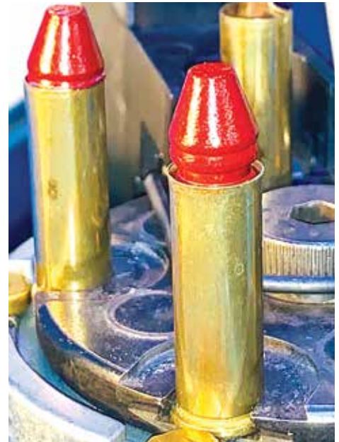
STATION 5 LEFT – BULLET INSERTED AND READY TO CRIMP; STATION 4 RIGHT – SLIGHTLY BELLED CASE WITH BULLET SITTING JUST INSIDE.
