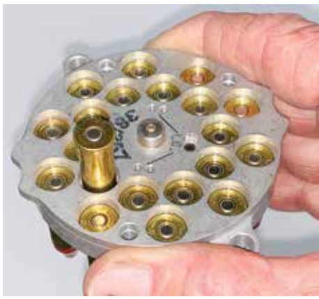
ST MACHINING LOADING BLOCK - CHECKS FOR SPLIT CASES, BAD CRIMPS, BENT RIMS, AND HIGH PRIMERS. THIS SPLIT CASE WON'T GO IN.
