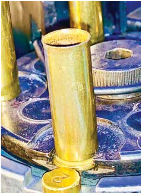
SLIGHTLY BELLED CASE ALLOWS BULLET TO SIT "INSIDE" CASE. OVERDOING IT SPLITS CASES. UNDERDOING IT CAUSES GOUGES IN BULLETS.
