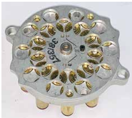
ST MACHINING LOADING BLOCK WITH TOP RING TURNED TO CHECK FOR HIGH PRIMERS. IT ALSO HOLDS ROUNDS IN PLACE TO USE AT THE LOADING TABLE.
